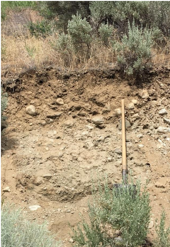
Figure 9. The Skaha soil series composed of glaciofluvial sands over gravels. The Skaha soils are the only soils in the sub-GI with a gravelly subsoil.
